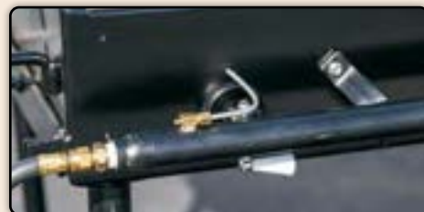
Gas Manifold With Cover Removed
